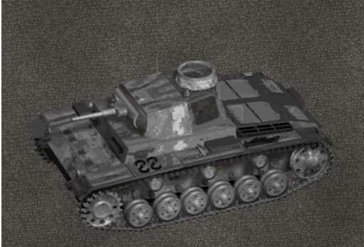
21--+LightMechanized-MLT light tank - pz.III ausf.f 37mm 2x 7.92 mg Panzerkampfwagen III (abbreviated PzKpfw III ) translating as "armoured battle vehicle
