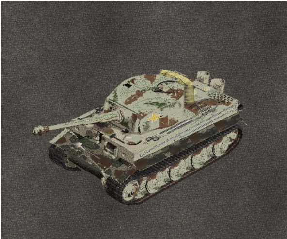
23--+HeavyMechanized-THT -VI Tiger pz VI tigerI ausf e 88mm gun 2xmg34 7.92 --Tiger I Ausf.E is a heavy tank It is armed with the powerful 8.8cm KwK36 L/56 main gun and two machineguns.--
